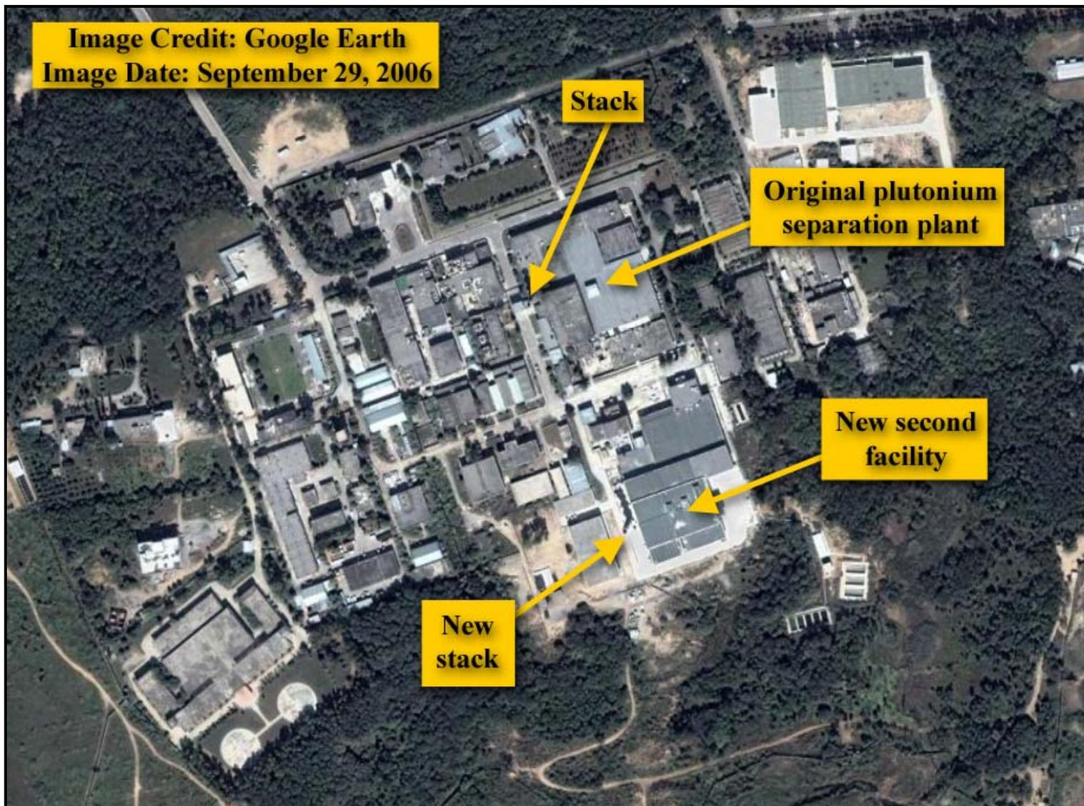
Figure 3. September 29, 2006 image of the New Labs site. The second facility appears to be finished. It has a stack just like the facility above it. The new facility appears to be a second plutonium separation plant.
