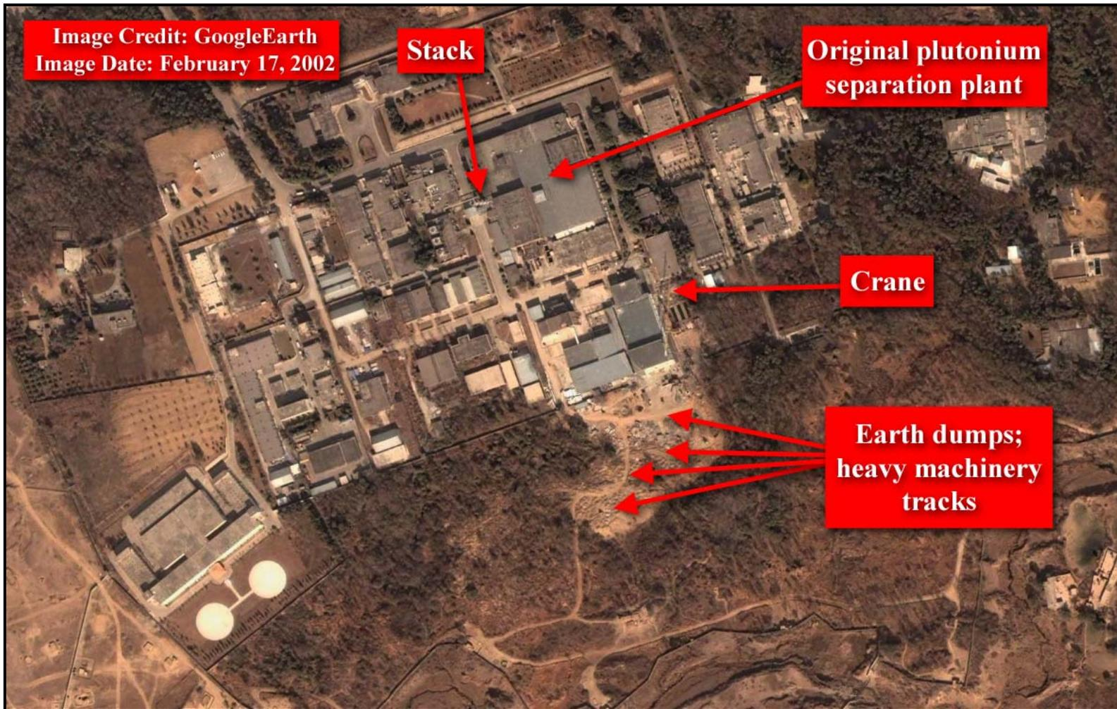
Figure 1. February 17, 2002 image of the New Labs facility at PINSTECH near Rawalpindi. The original plutonium separation plant with the stack can be seen. There is a crane and considerable construction activity with earth dumps and heavy machinery dirt tracks south of the original plutonium separation plant.
